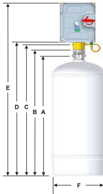
Figure 1. Dimensions of Cylinder Assembly with SVA and XV Control System
