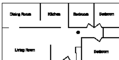
Figure 1: A SMOKE ALARM SHOULD BE LOCATED BETWEEN THE SLEEPING AREA AND THE REST OF THE FAMILY LIVING UNIT.
