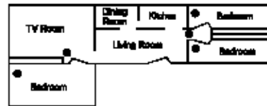
Figure 2: IN FAMILY LIVING UNITS WITH MORE THAN ONE SLEEPING AREA, A SMOKE ALARM SHOULD BE PROVIDED TO PROTECT EACH SLEEPING AREA IN ADDITION TO ALARMS REQUIRED IN BEDROOMS.
